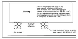
Figure A.6.4.3(4)(b) Separation Between Containers Less Than 40-25 ft (3-7.6 m). [Also change figure to show 25 ft (7.6 m) required separation.]
